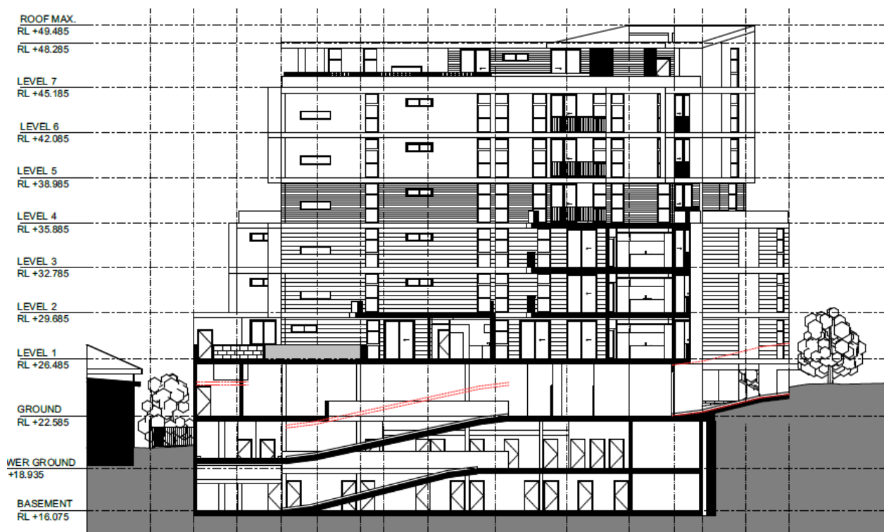
Figure 1. Elevation Schematic of the proposed superstructure showing the basement excavation (Extract from Holdsworth Design Section BB')
